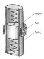
Fig. 1. An electromagnetic generator envisaged to generate UV radiation
