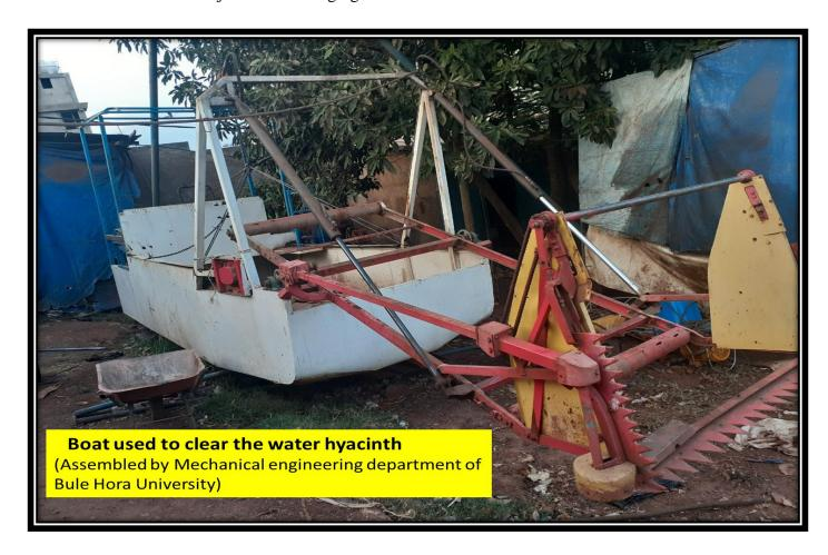
Fig. 4. A boat prepared to remove water hyacinth from Abaya Lake
